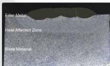
Single-layer welding seam tempered at 480 °C
