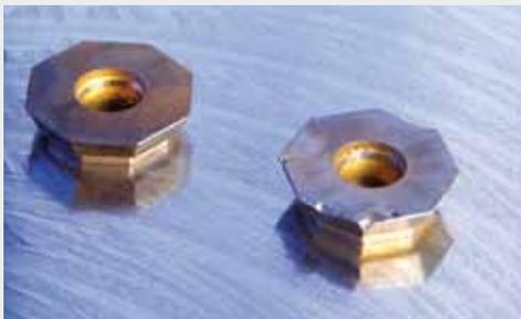
Both inserts were applied simultaneously with the same rotation speed at a high feed rate. With the left insert **ES ANTIKOR<sup>SL</sup>** was processed. The right insert was applied to conventional corrosion-resistant steel.
