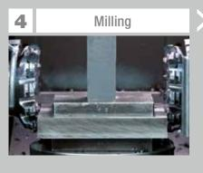
The blocks are machined on all six sides and the edges are neatly deburred.
