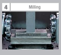
The blocks are machined on all six sides and the edges are neatly deburred.
