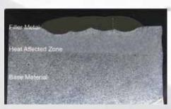
Single-layer welding seam tempered at 480  $^{\circ}\text{C}$
