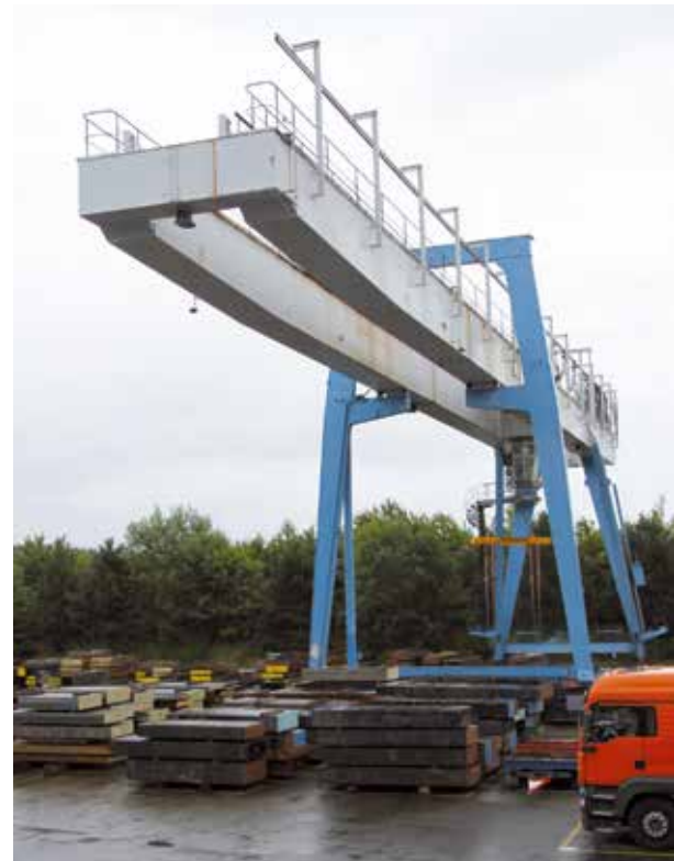
The gantry crane can lift up to 20 tons.
