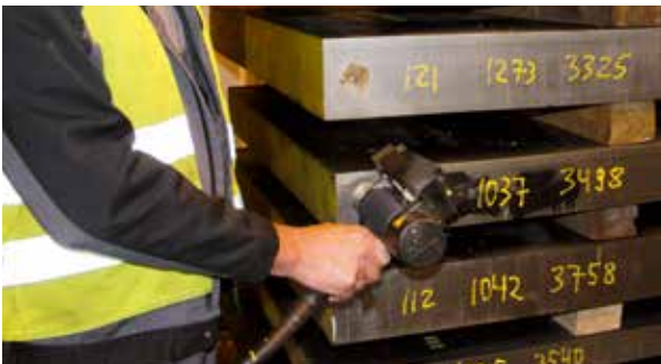
Stefan Lemmer inspects the quality of the steel with a mobile spectral analysis device.
