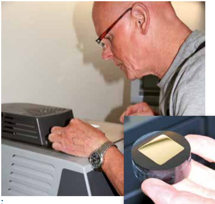
Hartmut Kemper inserts a piece of steel sawed to size into the mounting press, to produce a test specimen.
