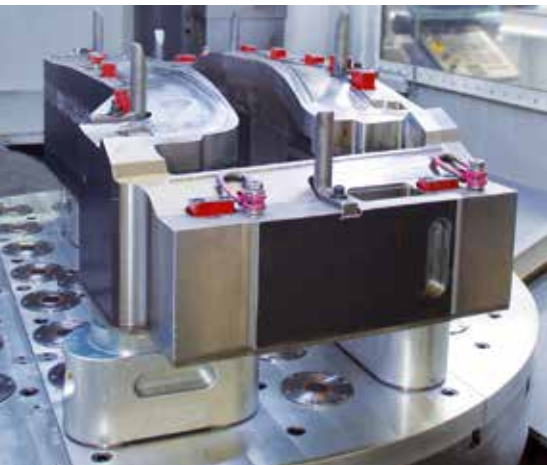
Five-sided machining with only a single reclamping procedure
