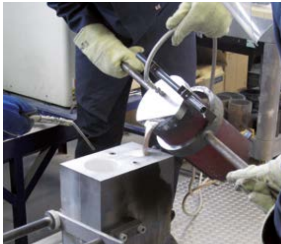
Pouring in the liquid aluminium
