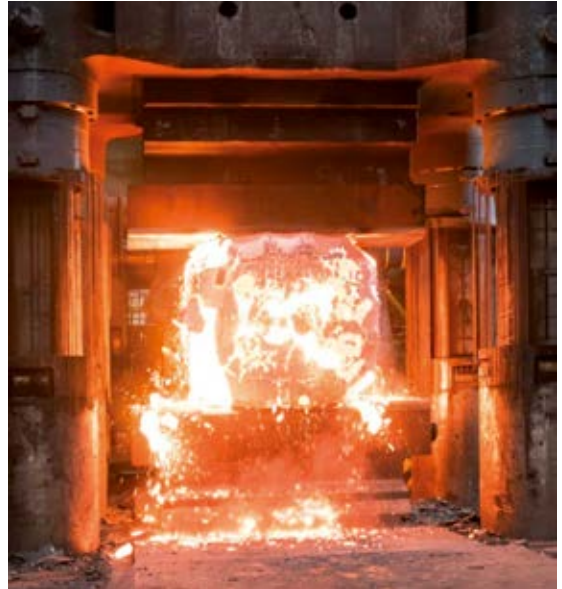
Stainless steels are produced in block formats weighing between 2.8 and 190 tonnes.
