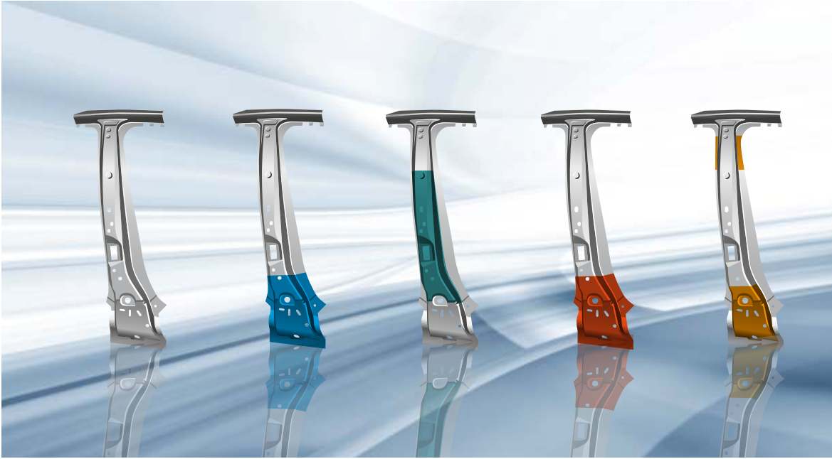
Tailored-property parts enhance the crash performance of vehicles
