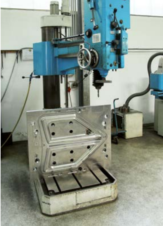
The mould for a car window seal is being produced here.
